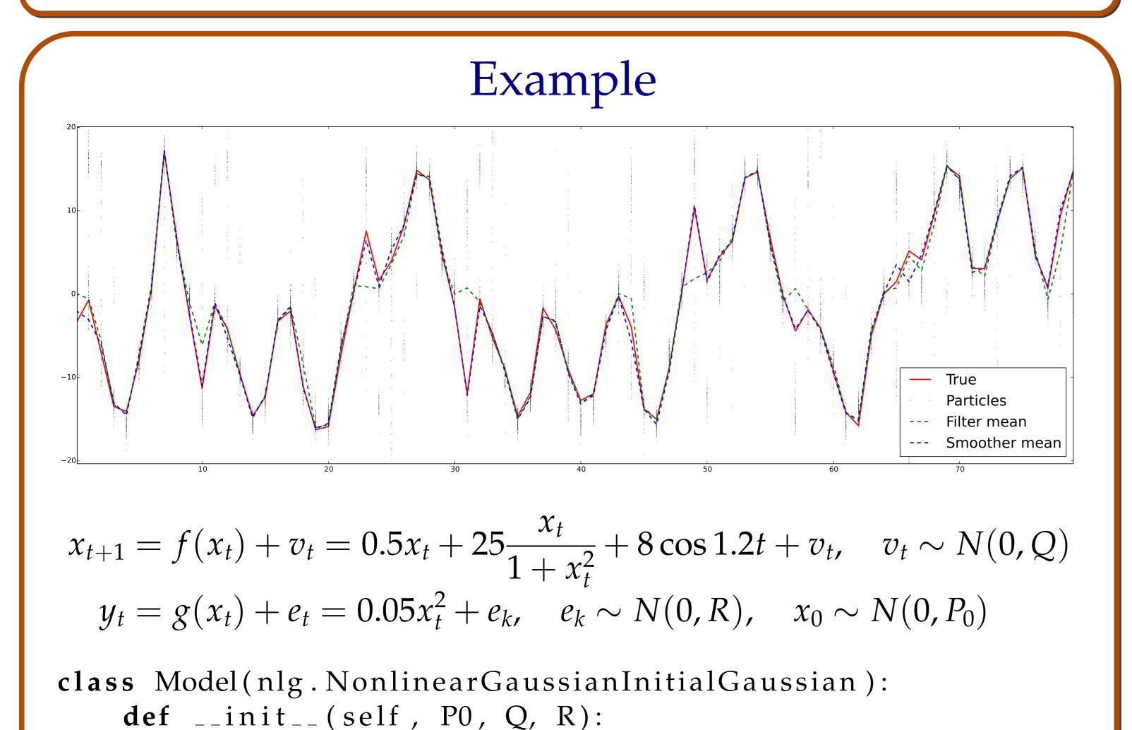
(a) For i = 1..Ni. Sample  $x_{t+1}^{(i)}$  from  $p(x_{t+1}|x_t^{(i)})$ ii. Set  $w_{t+1}^{(i)} = w_t^{(i)} p(y_{t+1}|x_{t+1}^{(i)})$ (b) Normalize weights,  $\hat{w}^{(i)} = w_{t+1}^{(i)} / \sum_j w_{t+1}^{(j)}$ (c) For i = 1..Ni. Sample  $x_{t+1}^{(i)} \sim p(x_{t+1}|y_{t+1})$  by drawing from the categorical distribution defined by  $(x_{t+1}^{(k)}, \hat{w}^{(k)}), k \in 1..N$ ii. Set  $w_{t+1}^{(i)} = \frac{1}{N}, i \in 1..N$
