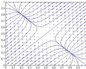
Figure 4.10: Interaction kernel (3.5) with  $\alpha = 0.58$ : antidiagonal equilibria locally stable.
