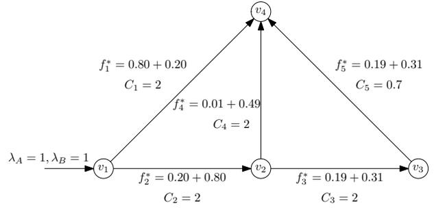
(a) Equilibrium flows for a simple network. All flows are less than edges capacities, so that the network is able to fully transfer the external inflows  $\lambda_A, \lambda_B$  to their destinations, node  $v_4$ .
