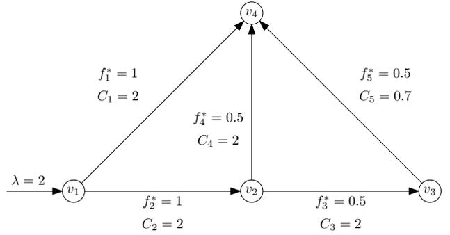
Fig. 2: A single-commodity network. The minimum residual capacity 0.2 is achieved at node  $v_3$ . Hence, under any perturbation of magnitude smaller than 0.2 the network is still be able to transfer the external inflow  $\lambda_{v_1}$  to the destination node  $v_4$ .
