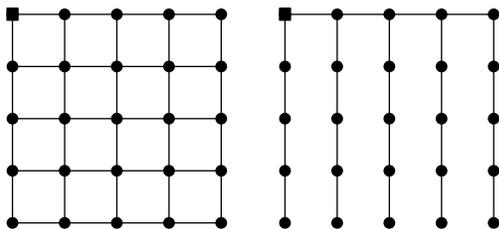
Fig. 4. On the left a square grid graph. On the right the correspondent spanning tree used in simulations. The square node is the anchor.
