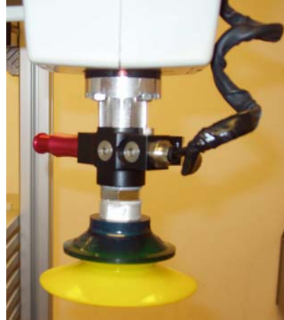
Figure 4.5 The suction cup mounted on the robot with an adapter attached in-between the robot and the suction cup.
