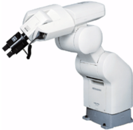
Figure 4.1 The Mitsubishi RV-2A, which is used in the project. Here with a gripper attached. 14
