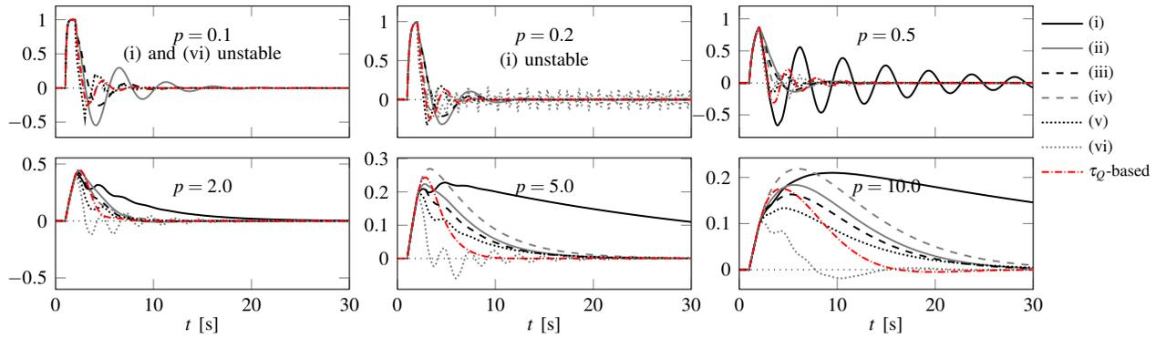
Fig. 6: Application of the proposed approach to class 4 in the benchmark: closed-loop responses of the controlled variable to a unit load disturbance step.
