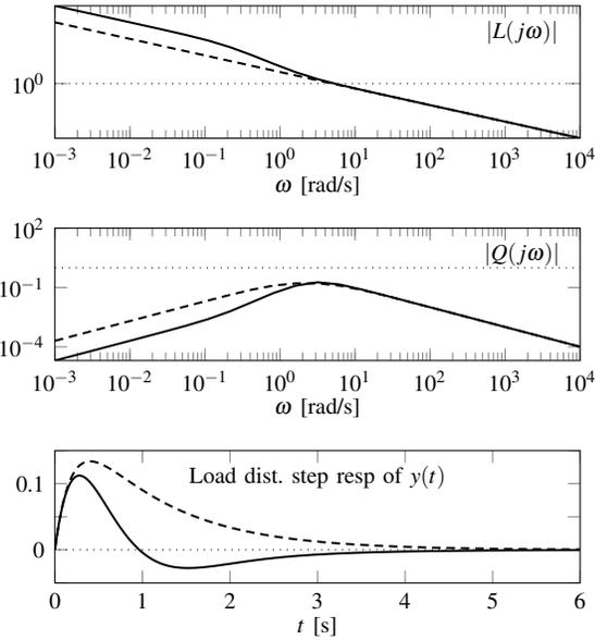
Fig. 3: Introductory example illustrating the proposed approach *rationale*: cancellation-based PI (dashed plots) and the same PI augmented with a pole-zero couple (solid plots).
