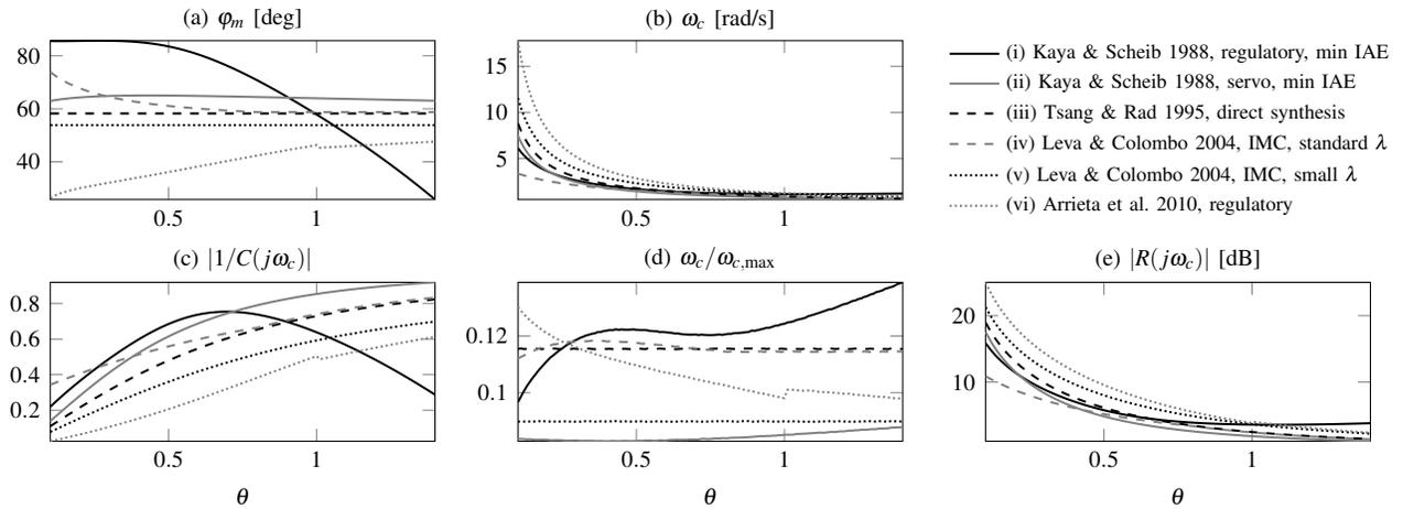
Fig. 2: Behaviour of some PID tuning rules for FOPDT models in the light of the ideas of Section III.
