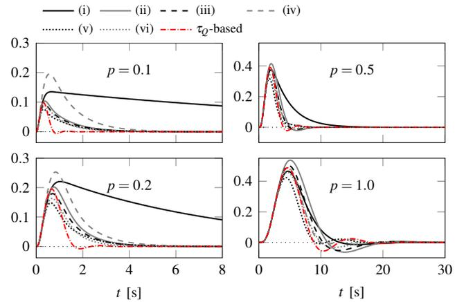
Fig. 5: Application of the proposed approach to class 2 in the benchmark: closed-loop responses of the controlled variable to a unit load disturbance step.
