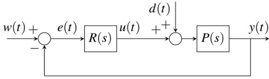
Fig. 1: Typical control loop with load disturbance.
