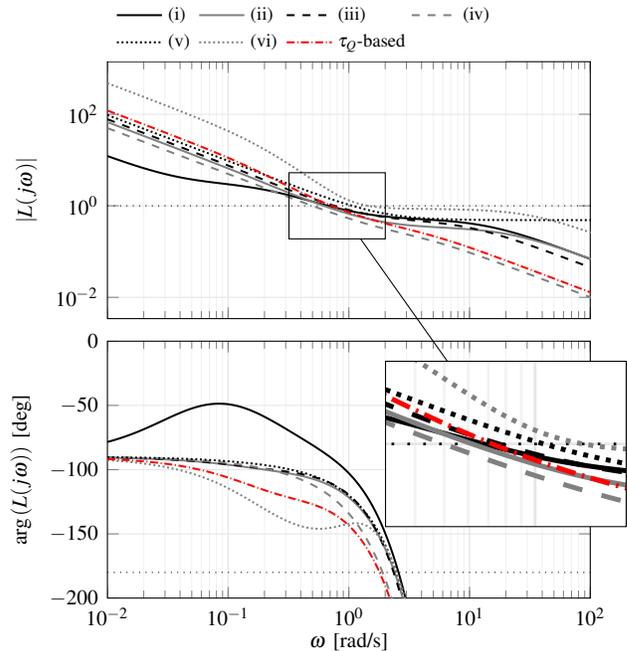
Fig. 7: Bode diagram of the open-loop transfer function  $L(s)$  with class 4 for  $p = 5$ .
