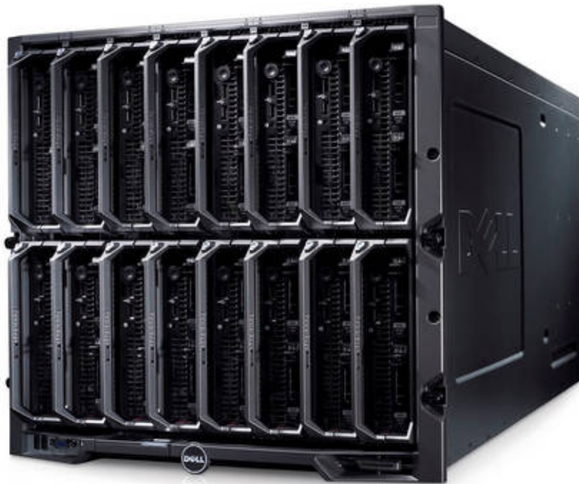
Figure 3.8: Dell PowerEdge M1000e blade system, fully populated by half-height blades
