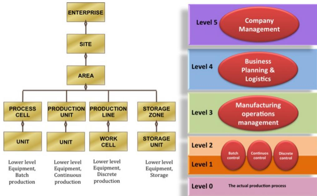
**Figur 1** The physical hierarchy (left) and functional hierarchy (right) of the PERA model.
