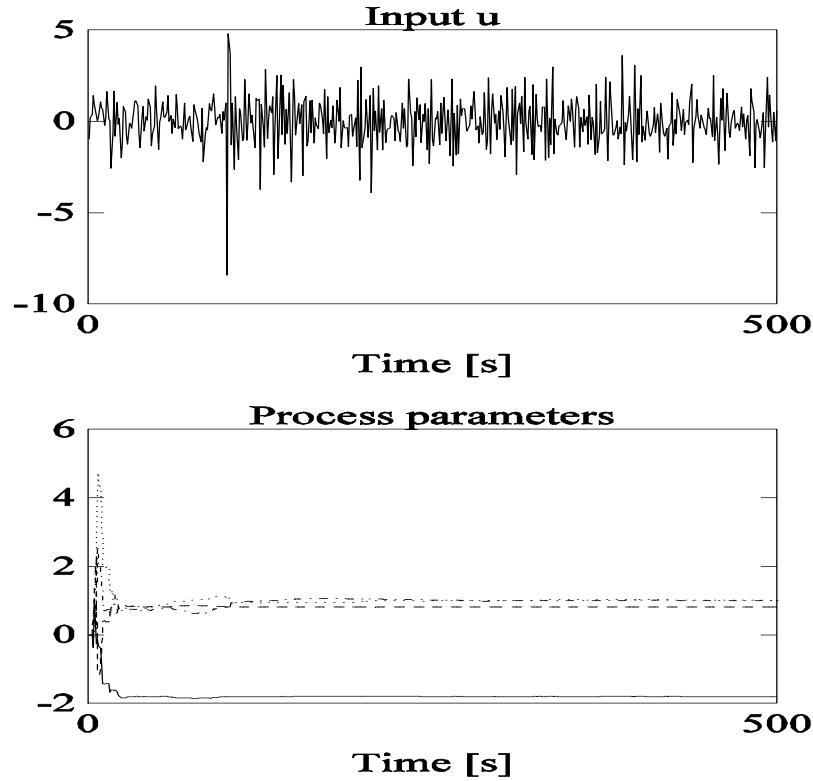
Indirect adaptive control. The second-order process is controlled by an output feedback control law with pole assignment to the origin  $z=0$ . The histories of the input  $u$ , output  $y$ , and the estimated process parameters and the controller parameters are displayed.
