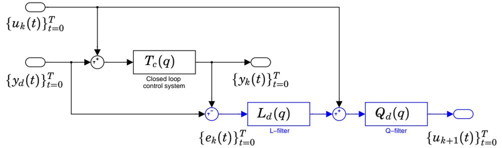
**Figure 2** ILC setup: The update of the correction signal sequence  $\{u_{k+1}\}$  is made in batch after each run.
