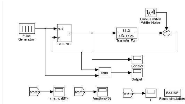
**Figure 5** Simulink model *stupidDCsim* used for simulation of STUPID-controlled DC-servo.
