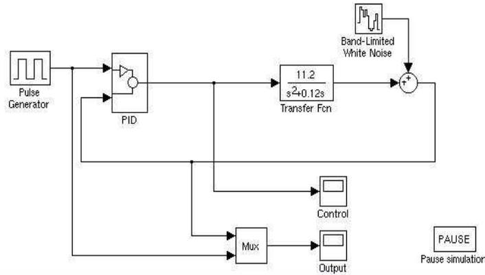
**Figure 4** Simulink model *pidDCsim* used for simulation of fixed-PID-controlled DC-servo.
