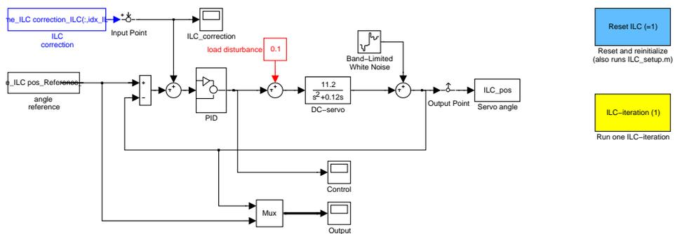
**Figure 6** Simulation model *ILC\_pidDCsim* using Iterative Learning Control (ILC) for improving reference following.
