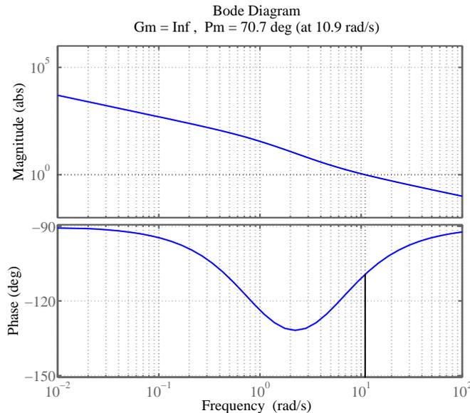
**Figure 3** Margin plot for the open loop system in problem 2b.
