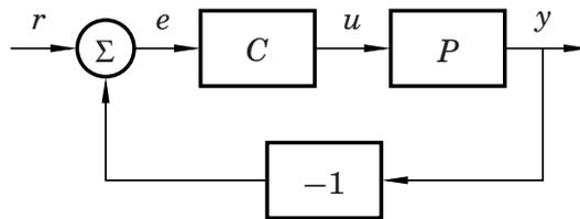
**Figure 4** Block diagram of the closed-loop system in Problem 4.
