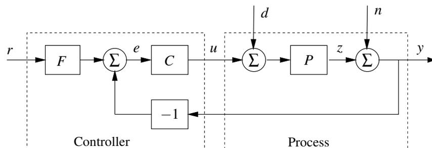
Figure 3 2-DOF controller structure in Problem 4.
