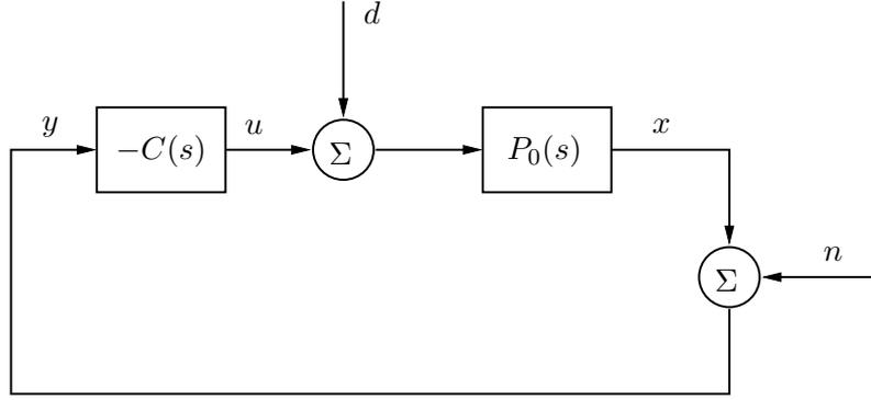
**Figure 5** Block diagram of the closed-loop system in Problem 7.
