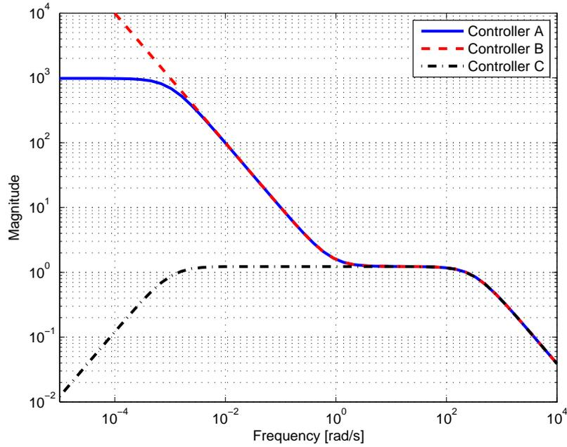
**Figure 4** Bode diagram of three possible candidates for the LQG controller in Problem 6.
