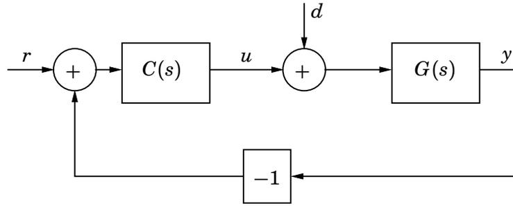
**Figure 3** The closed loop control system in Problem 4.
