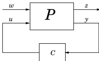
**Figure 11.2** General closed-loop system in Problems 11.1 and 11.2.
