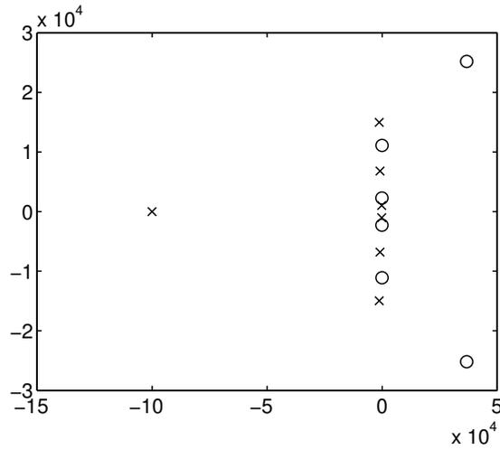
Figure 6.2 Pole-zero configuration of a resonant mechanical system.
