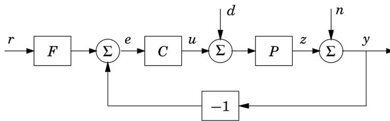
Figure 6.3 Two degree of freedom controller structure.
