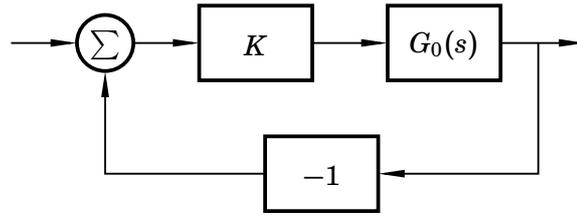
Figure 1.5 Simple control loop
