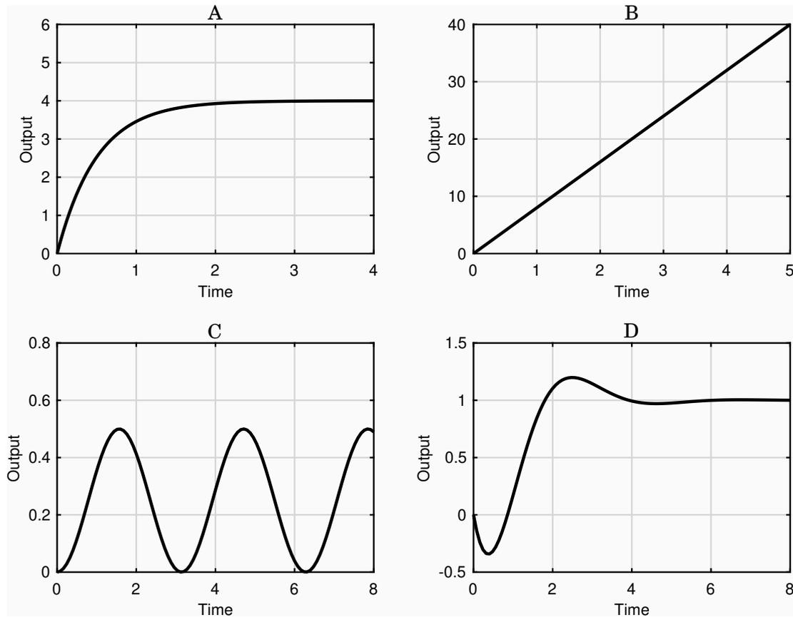
Figure 1.1 Step responses of four linear systems.
