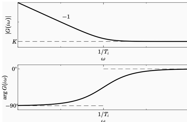
**Figure 1.2** Bode diagram of  $G(s) = K\left(1 + \frac{1}{sT_i}\right)$
