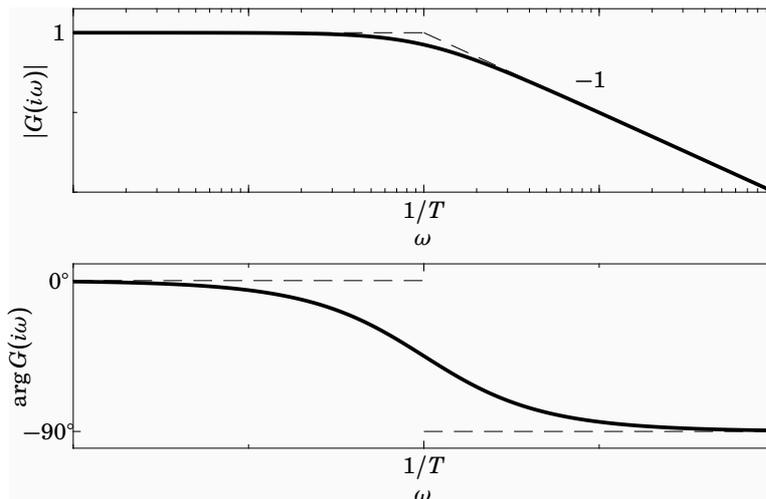
**Figure 1.1** Bode diagram of  $G(s) = \frac{1}{1+sT}$
