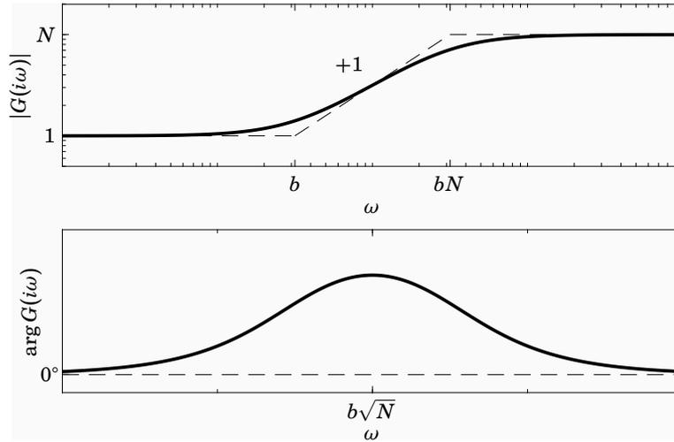
**Figure 1.3** Bode diagram of  $G(s) = \frac{N(s+b)}{s+bN}$
