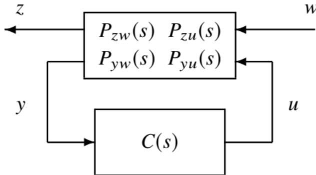
Closed-loop transfer function from  $w$  to  $z$ :
