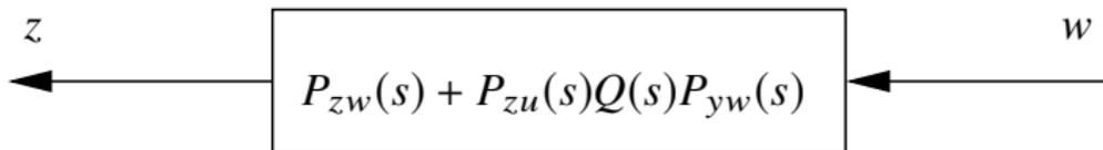
Once  $Q(s)$  has been designed, the corresponding controller can be found.
