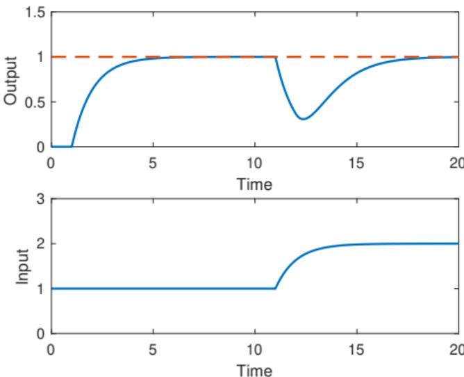
Looks perfect. But do not forget the fundamental limitation imposed by the time delay! Respect the rule of thumb  $\omega_c < \frac{1.6}{L}$  when designing  $C_0$ .
