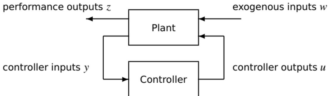
The choice of controller corresponds to designing a transfer matrix  $Q(s)$ , to get desirable properties of the following map from  $w$  to  $z$ :
