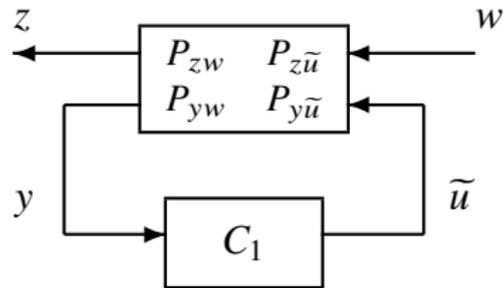
If  $P_0(s)$  is unstable, let  $C_0(s)$  be some stabilizing controller. Then the previous argument can be applied with  $P_{zw}$ ,  $P_{z\tilde{u}}$ ,  $P_{yw}$ , and  $P_{y\tilde{u}}$  representing the stabilized system.
