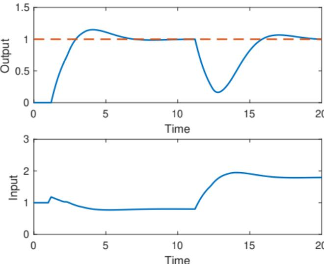
Performance degradation due to model and plant mismatch.
