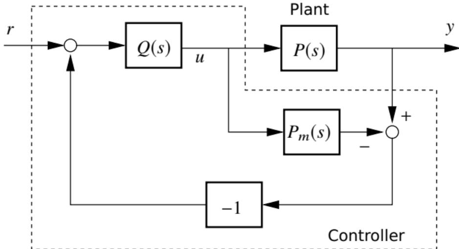
(Negative) Feedback is used only if the real plant  $P(s)$  deviates from the model  $P_m(s)$ .  $Q(s)$ ,  $P(s)$ ,  $P_m(s)$  must be stable.
