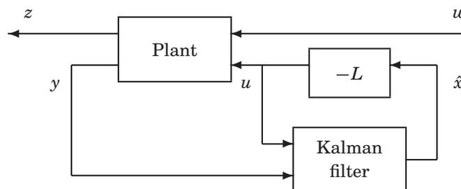
**Figure 11.1** An optimal output feedback controller—an LQG controller—consists of an optimal state feedback  $-L$  from an optimal state estimate  $\hat{x}$  (given by a Kalman filter).
