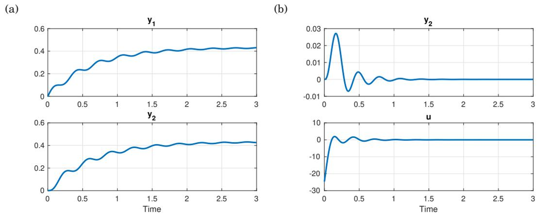
**Figure 11.2** Flexible servo example: (a) Open-loop impulse response, (b) first design iteration.
