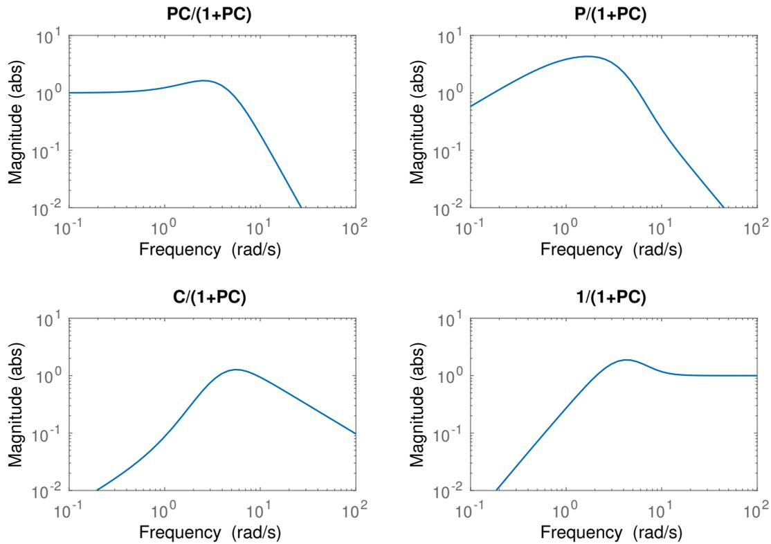
Figure 11.7 “Gang of four” for the LQG controller with integral action
