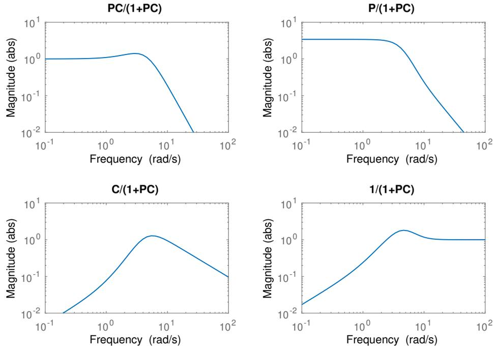
**Figure 11.6** “Gang of four” for the LQG-controlled DC servo.
