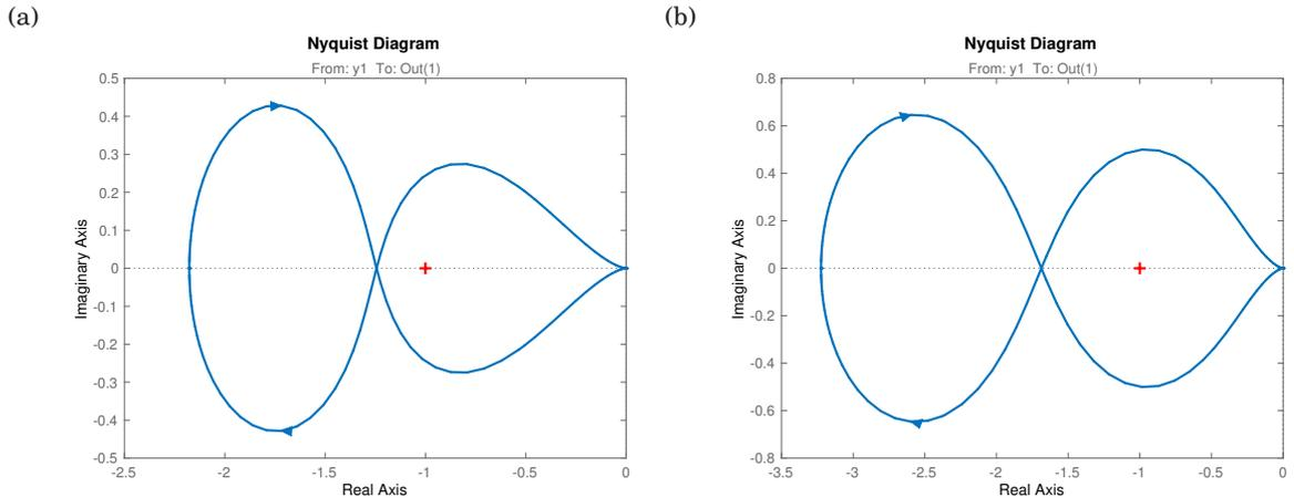
Figure 11.4 Doyle–Stein example: (a) Original example (b) Example with loop transfer recovery.
