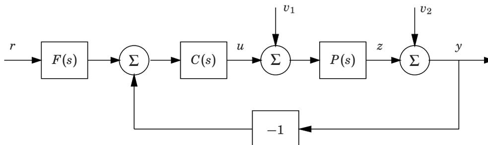
**Figure 11.5** Basic control loop for LQG control of a DC servo.
