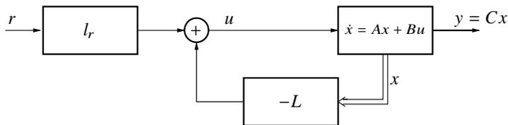
If the system  $(A, B)$  is *controllable* then we can place the eigenvalues of  $(A - BL)$  arbitrarily
