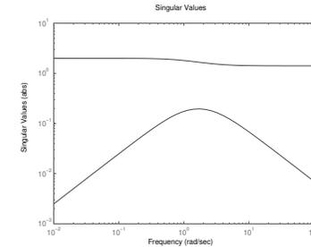
The largest singular value of  $G(i\omega) = \begin{bmatrix} \frac{1}{i\omega+1} & 1 \\ \frac{1}{i\omega+2} & 1 \end{bmatrix}$  is fairly constant. This is due to the second input. The first input makes it possible to control the difference between the two tanks, but mainly near  $\omega = 1$  where the dynamics make a difference.
