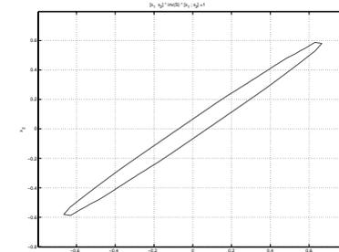
Plot of  $\begin{bmatrix} x_1 & x_2 \end{bmatrix} \cdot W_c^{-1} \begin{bmatrix} x_1 \\ x_2 \end{bmatrix} = 1$  corresponds to the states we can reach by  $\int_0^\infty |u(t)|^2 dt = 1$ .
