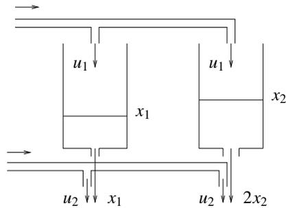
$$\begin{aligned} \dot{x}_1 &= -x_1 + u_1 & y_1 &= x_1 + u_2 \\ \dot{x}_2 &= -2x_2 + u_1 & y_2 &= 2x_2 + u_2 \end{aligned}$$
