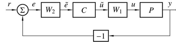
Select decoupling filters  $W_1$  (input decoupling) and/or  $W_2$  (output decoupling) so that the controller sees a diagonal plant:
