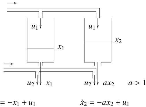
$$G(s) = \begin{bmatrix} \frac{1}{s+1} & 1 \\ \frac{2}{s+2} & 1 \end{bmatrix}. \quad \text{Find zero from } \det G(s) = \frac{-s}{(s+1)(s+2)}$$
