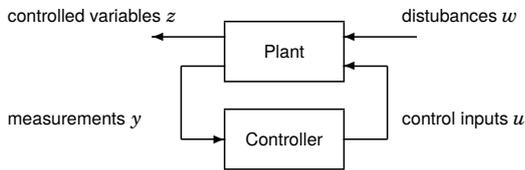
The choice of controller corresponds to designing a transfer matrix  $Q(s)$ , to get desirable properties of the following map from  $w$  to  $z$ :
