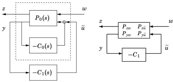
If  $P_0(s)$  is unstable, let  $C_0(s)$  be some stabilizing controller. Then the previous argument can be applied with  $P_{zw}$ ,  $P_{z\tilde{u}}$ ,  $P_{yw}$ , and  $P_{y\tilde{u}}$  representing the stabilized system.
