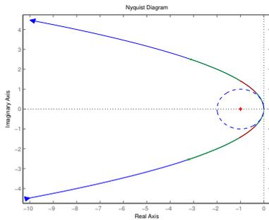
The distance from the loop gain  $L(i\omega I - A)^{-1}B$  to  $-1$  is never smaller than 1. This is always true(!) when  $Q_1 > 0$ ,  $Q_{12} = 0$  and  $Q_2 > 0$  is scalar. The phase margin is at least  $60^\circ$  and the gain margin is infinite!
