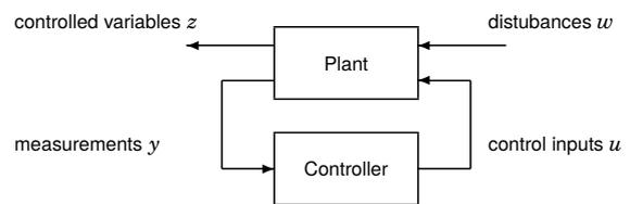
The objective is to find a controller that optimizes the transfer matrix  $G_{zw}(s)$  from disturbances (and setpoints)  $w$  to controlled outputs  $z$ .
