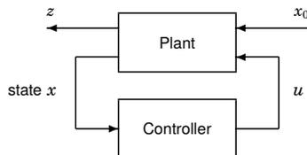
$$\text{Minimize } J = z^2 = \int_0^\infty \begin{pmatrix} x(t) \\ u(t) \end{pmatrix}^T \begin{pmatrix} Q_1 & Q_{12} \\ Q_{12}^T & Q_2 \end{pmatrix} \begin{pmatrix} x(t) \\ u(t) \end{pmatrix} dt$$
