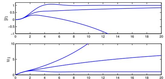
The second controller has a major impact on the first loop! Gain reversal in  $u_1 \rightarrow y_1$  when  $K_2 = 1.6$ .
