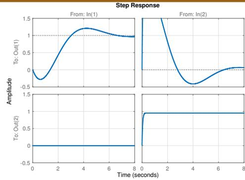
The RHP zero does not prevent a fast  $y_2$  response to  $r_2$  but at the price of a simultaneous undesired response in  $y_1$ .
