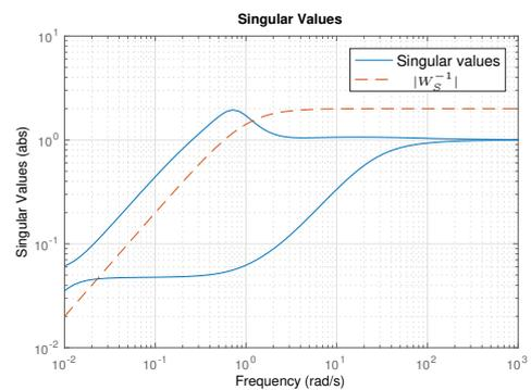
$W_S(s) = \frac{s+1}{2s}$ , impossible to meet due to RHP zero
