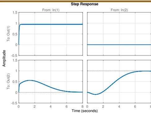
The RHP zero does not prevent a fast  $y_1$  response to  $r_1$  but at the price of a simultaneous undesired response in  $y_2$ .
