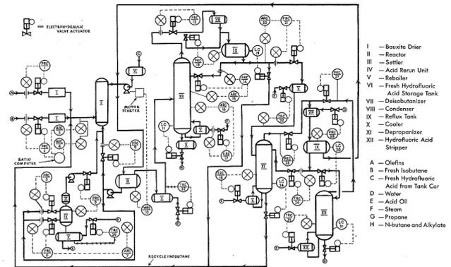
Figure 13-6. Automatic control system for Perco motor fuel alkylation process.
