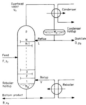
Raw oil inserted at bottom; different petro-chemical subcomponents extracted
