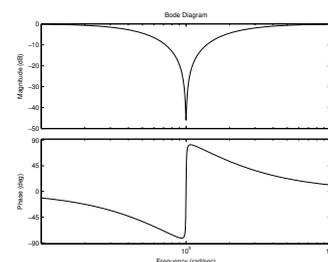
(E.g., suppress measurement noise at specific frequency)
