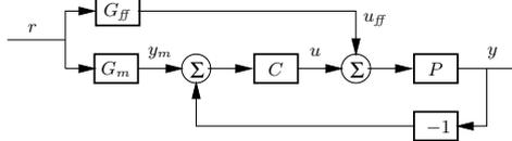
$G_m$  and  $G_{ff}$  can be viewed as generators of the desired output  $y_m$  and the feedforward  $u_{ff}$  that corresponds to  $y_m$
