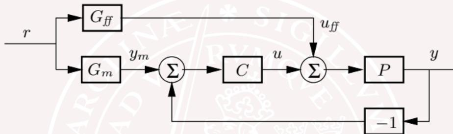
$G_m$  and  $G_{ff}$  can be viewed as generators of the desired output  $y_m$  and the feedforward  $u_{ff}$  that corresponds to  $y_m$
