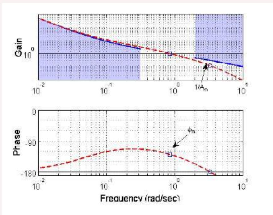
Approximations are inexact around cross-over frequency  $\omega_c$ . In this region, focus is on stability margins ( $A_m, \varphi_m$ )
