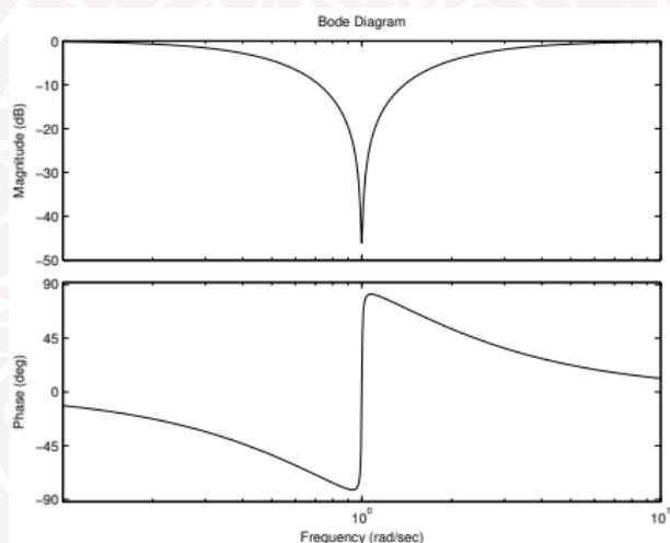
(E.g., suppress measurement noise at specific frequency)
