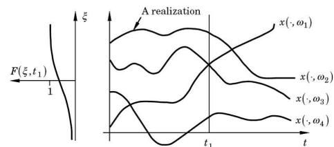
For a **Gaussian process**,  $x(t_1, \cdot)$  has a normal distribution
