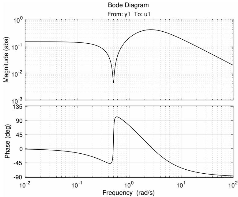
**Figure 9.3** LQG controller Bode diagram in Problem 9.4 c.
