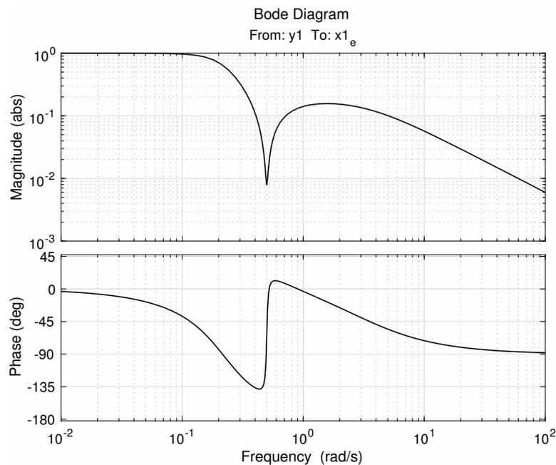
**Figure 9.2** Kalman filter Bode diagram in Problem 9.4 b.
