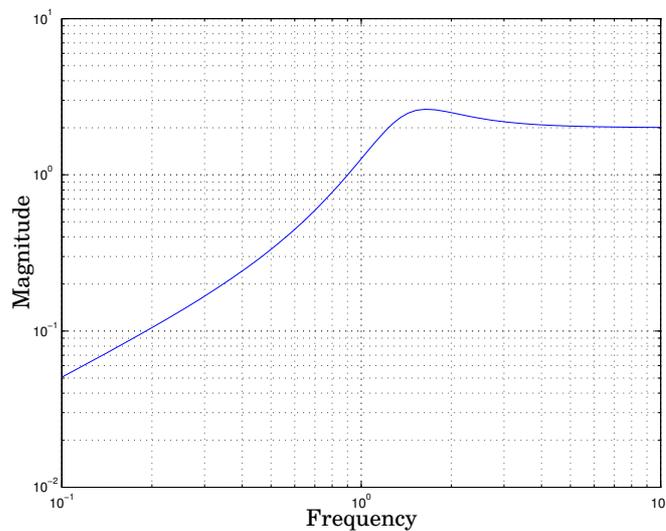
**Figure 3.2** Bode magnitude diagram for  $G_{vn}(s)$ .
