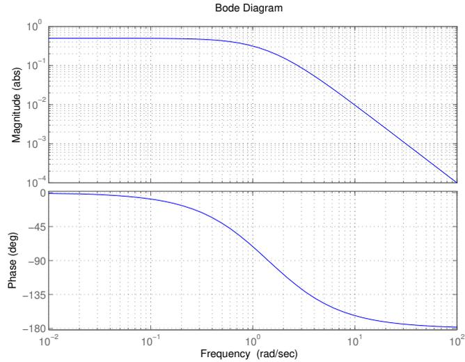
Figure 2.4 Bode diagram for  $P(s)$  in Problem 2.5.
