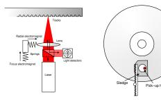
The pick-up-head has two electromagnets for fast positioning of the lens (left). Larger radial movements are taken care of by the sledge (right).
