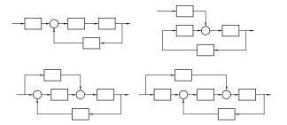
For linear systems, all of these structures are equivalent
