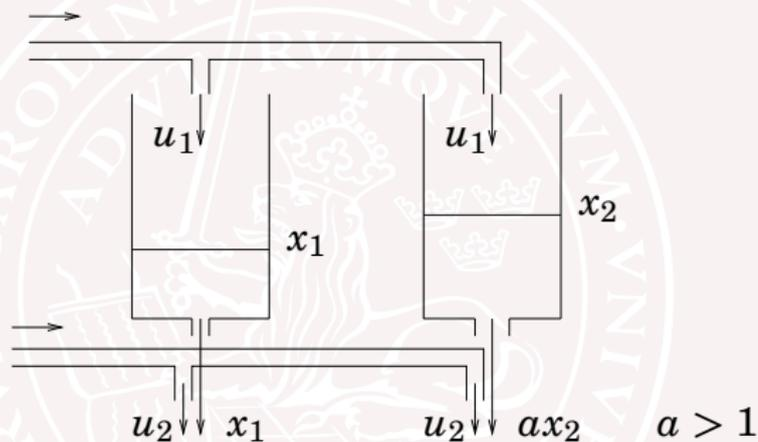
$$\begin{aligned}\dot{x}_1 &= -x_1 + u_1 & \dot{x}_2 &= -ax_2 + u_1 \\ y_1 &= x_1 + u_2 & y_2 &= ax_2 + u_2\end{aligned}$$
