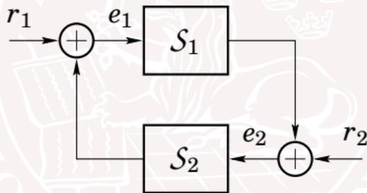
Assume that  $\mathcal{S}_1$  and  $\mathcal{S}_2$  are input-output stable. If  $\|\mathcal{S}_1\| \cdot \|\mathcal{S}_2\| < 1$ , then the gain from  $(r_1, r_2)$  to  $(e_1, e_2)$  in the closed loop system is finite.
