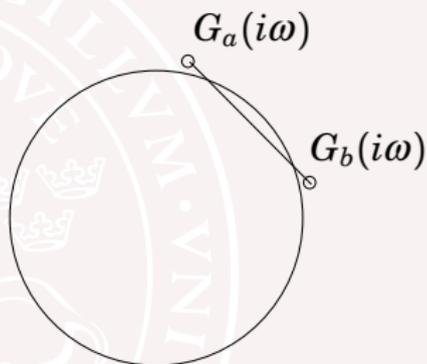
An lower bound  $|G(i\omega_i)|$  is a *non-convex* quadratic constraint. This should be avoided in optimization.
