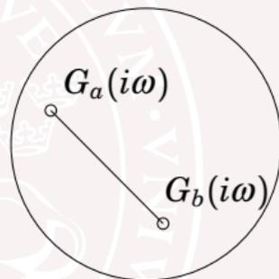
An amplitude bound  $|G(i\omega_i)| < c$  is a quadratic constraint.
