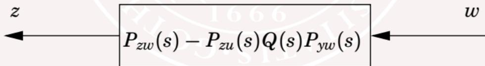
Once  $Q(s)$  is determined, a corresponding controller is derived.
