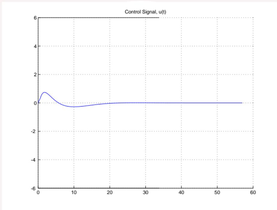
The step input stays within its amplitude bound  $|u(t)| \leq 6$ .
