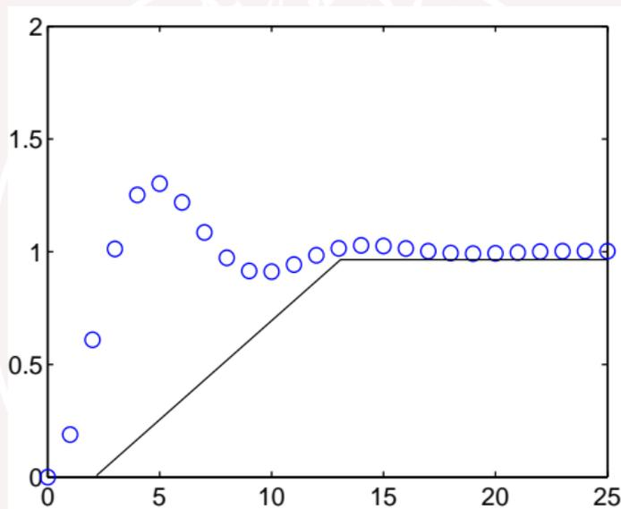
The step response depends linearly on  $Q_k$ , so every time  $t_k$  with a lower bound gives a linear constraint.
