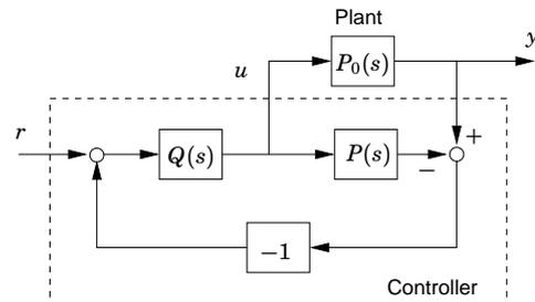
Feedback is used only as the real process deviates from  $P(s)$ .
