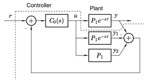
The Smith predictor uses an internal model of the process (with and without the delay). Ideally  $Y$  and  $Y_1$  cancel each other and only feedback from  $Y_2$  "without delay" is used.
