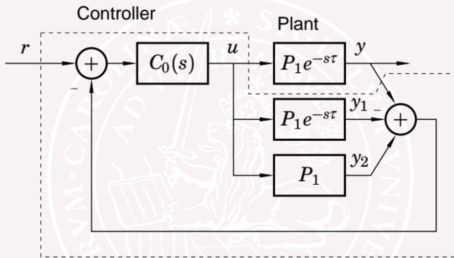
The Smith predictor uses an internal model of the process (with and without the delay). Ideally  $Y$  and  $Y_1$  cancel each other and only feedback from  $Y_2$  “without delay” is used.
