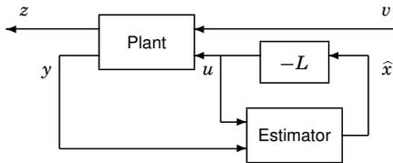
$$\begin{aligned} \text{Plant:} \quad & \begin{cases} \dot{x}(t) = Ax(t) + Bu(t) + v_1(t) \\ y(t) = Cx(t) + v_2(t) \end{cases} \\ \text{Controller:} \quad & \begin{cases} \frac{d}{dt}\hat{x}(t) = A\hat{x}(t) + Bu(t) + K[y(t) - C\hat{x}(t)] \\ u(t) = -L\hat{x}(t) \end{cases} \end{aligned}$$
