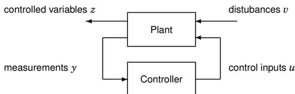
For a linear plant, let  $v$  be white noise of intensity  $R$ . Find a controller that minimizes the output variance:
