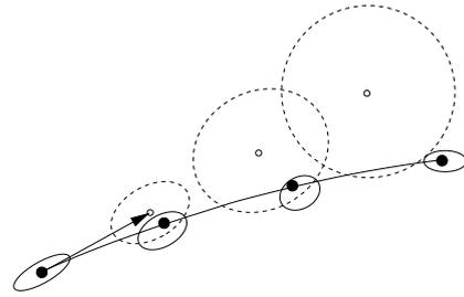
Dotted ellipses show estimates based on only a model with known initial state. Solid ellipses show Kalman filter estimates based on noisy measurements.
