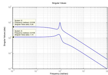
Figure: The singular values of the transfer function matrix (prev slide). Note that  $G(0)=\begin{bmatrix} 2 & 4 \\ 0 & 3 \end{bmatrix}$  which corresponds to  $M$  in the SVD-example above.  $\|G\|_\infty = 10.3577$ .
