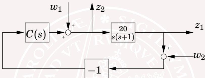
We previously minimized  $\int_{-\infty}^{\infty} G_{zw}(i\omega)G_{zw}(i\omega)^*d\omega$  subject to step response bounds on the transfer functions from  $w_1$  and  $w_2$  to  $z_1$ :
