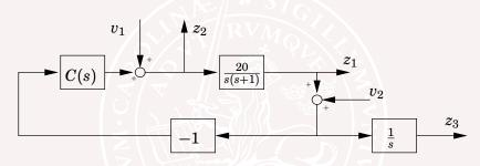
The transfer matrix from  $(v_1, v_2)$  to  $(z_1, z_2, z_3)$  is
