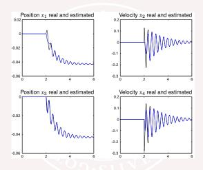
The measurement  $y_1$  is not trusted, so the estimate of  $x_1$  slows down.
