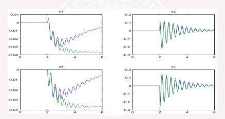
When only velocity is penalized, a static position error remains
