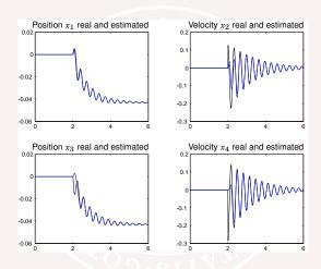
The measurement  $y_2$  is not trusted, so the estimate of  $x_3$  slows down.
