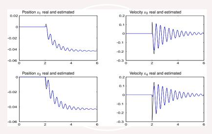
A Kalman filter estimates the states using measured positions.
