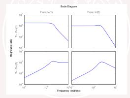
Nonzero static gain in  $\frac{P}{1+PC}$  indicates poor disturbance rejection
