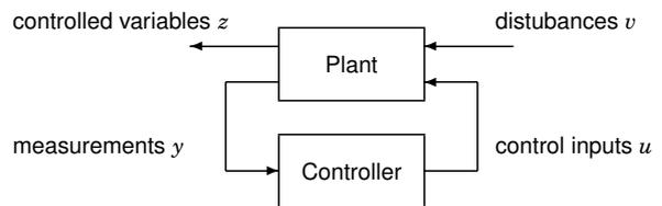
For a linear plant, let  $v$  be white noise of unit intensity. Find a controller that minimizes the output variance:
