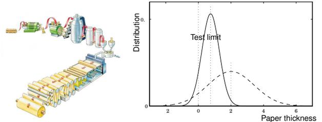
All paper production below the test limit is wasted.
