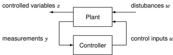
The objective is to find a controller that optimizes the transfer matrix  $G_{zw}(s)$  from disturbances  $w$  to controlled outputs  $z$ .
