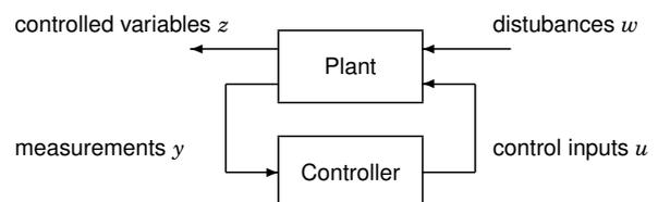
For a linear plant, minimize a quadratic function of the map from disturbance  $w$  to controlled variable  $z$
