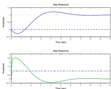
Figure : Closed loop step responses with controller  $C_2(s)$  for the two outputs  $y_1$  (solid) and  $y_2$  (dashed). The right half plane zero does not prevent a fast  $y_2$ -response to  $r_2$  but at the price of a simultaneous undesired response in  $y_1$ .
