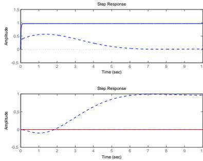
Figure : Closed loop step responses with controller  $C_3(s)$  for the two outputs  $y_1$  (solid) and  $y_2$  (dashed). The right half plane zero does not prevent a fast  $y_1$ -response to  $r_1$  but at the price of a simultaneous undesired response in  $y_2$ .
