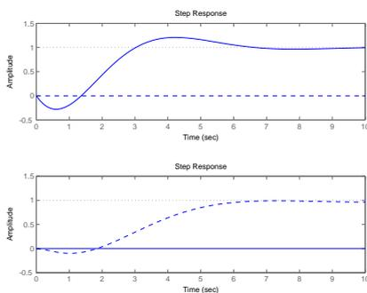
Figure : Closed loop step responses with decoupling controller  $C_1(s)$  for the two outputs  $y_1$  (solid) and  $y_2$  (dashed). The upper plot is for a reference step for  $y_1$ . The lower plot is for a reference step for  $y_2$ .
