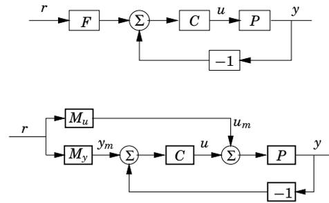
For linear systems all 2DOF configurations have the same properties. For the systems above we have
