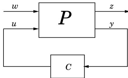
Figure 11.2 General form of a closed loop system.
