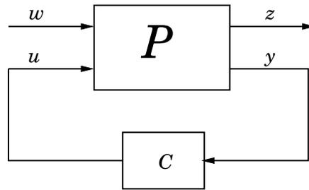
**Figure 11.5** General form of a closed loop system.
