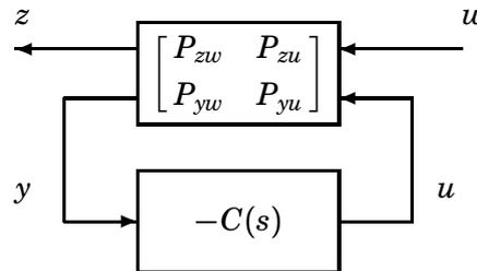
**Figure 14.4** General form of a closed loop system.
