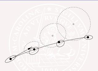
Dotted ellipses show estimates based on only a model with known initial state. Solid ellipses show Kalman filter estimates based on noisy measurements.
