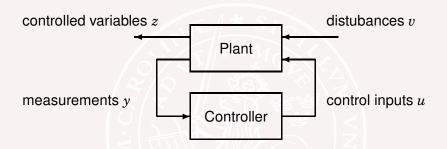
For a linear plant, minimize a quadratic function of the map from disturbance v to controlled variable z
