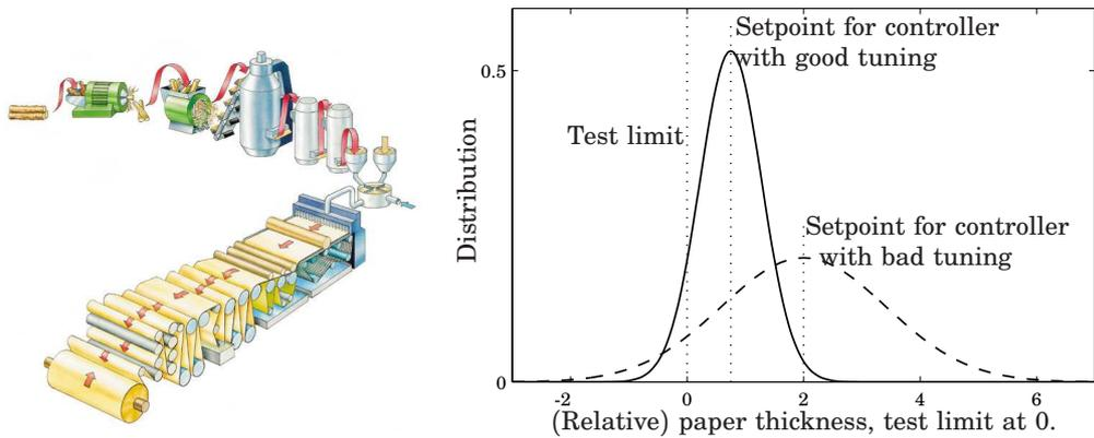
**Figure 3.3** To be of acceptable quality, products must exceed a certain threshold. By minimizing the variance of the thickness we see that the average of the paper thickness can be reduced significantly ( we come closer to the test limit) for the same yield. This may save a lot in production costs regarding both energy and raw material.
