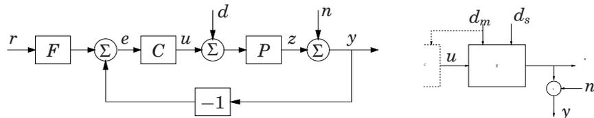
**Figure 3.2** *(Left)* The basic control loop with load disturbances  $d$  and measurement noise  $n$ . *(Right)* Load disturbances which can be measured,  $d_m$ , e.g., changes in outer temperature, can be (partially) compensated for by feedforward to the control signal.
