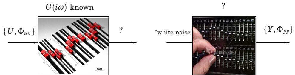
**Figure 3.1** Illustration of two main questions of disturbance modelling in this chapter; *(left)* What is the output spectral density  $\Phi_{yy}$  given that we know the input spectral density  $\Phi_{uu}$  and and the linear filter  $G(i\omega)$ ? *(right)* Knowing the output spectral density, find a stable linear filter which gives the same output spectral density if fed by white noise.
