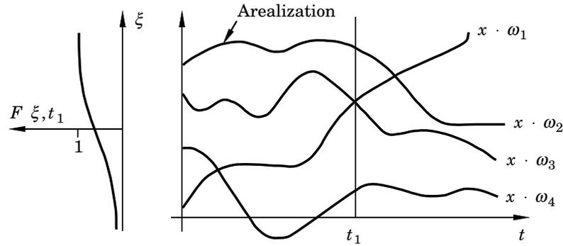
**Figure 3.4** A stochastic process: For a fixed  $\omega$  we call it a realization, for fixed time  $t_1$  it will correspond to a random variable with a distribution  $F(\xi, t_1) = \text{Prob}\{x(t_1) \leq \xi\}$ .
