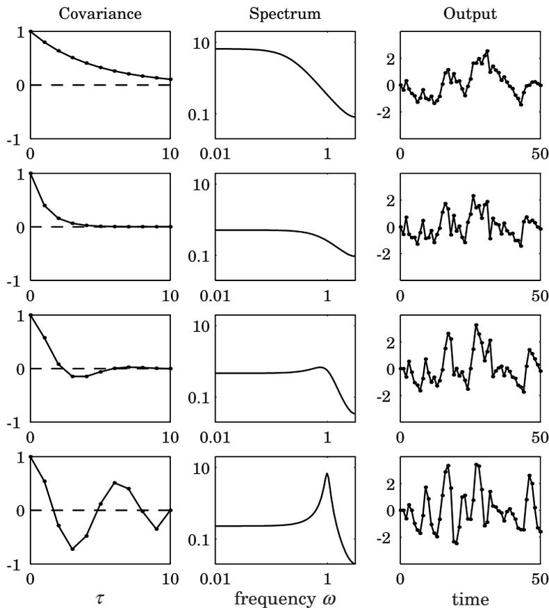
**Figure 3.5** Relations between covariance function, spectral density and a typical realization.
