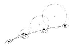
Dotted ellipses show estimates based on only a model with known initial state. Solid ellipses show Kalman filter estimates based on noisy measurements.
