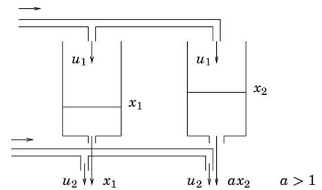
$$\begin{aligned} \dot{x}_1 &= -x_1 + u_1 & y_1 &= x_1 + u_2 \\ \dot{x}_2 &= -ax_2 + u_1 & y_2 &= ax_2 + u_2 \end{aligned}$$
