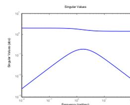
The largest singular value of  $G(i\omega) = \begin{bmatrix} \frac{1}{i\omega+1} & 1 \\ \frac{2}{i\omega+2} & 1 \end{bmatrix}$  is fairly constant. This is due to the second input. The first input makes it possible to control the difference between the two tanks, but mainly near  $\omega = 1$  where the dynamics make a difference.
