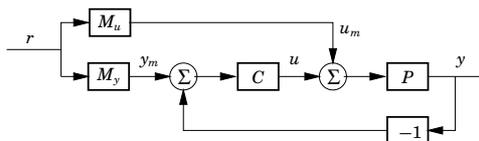
Notice that  $M_u$  and  $M_y$  can be viewed as generators of the desired output  $y_m$  and the inputs  $u_m$  which corresponds to  $y_m$ .
